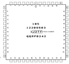
mask number references the photo mask used to fabricate the silicon chip inside the package. The mask number will cross reference
