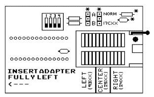
NOTE: The 10K\* resistor and .0022uF\* capacitor on the upper right corner of the adapter board are optional and only required to support the early PCD8572 serial eeprom from Microchip.
